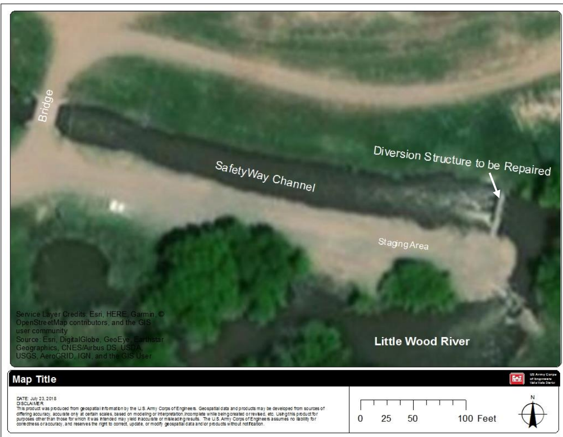
Figure 1-2. Aerial view of the diversion structure and the safety way channel.
