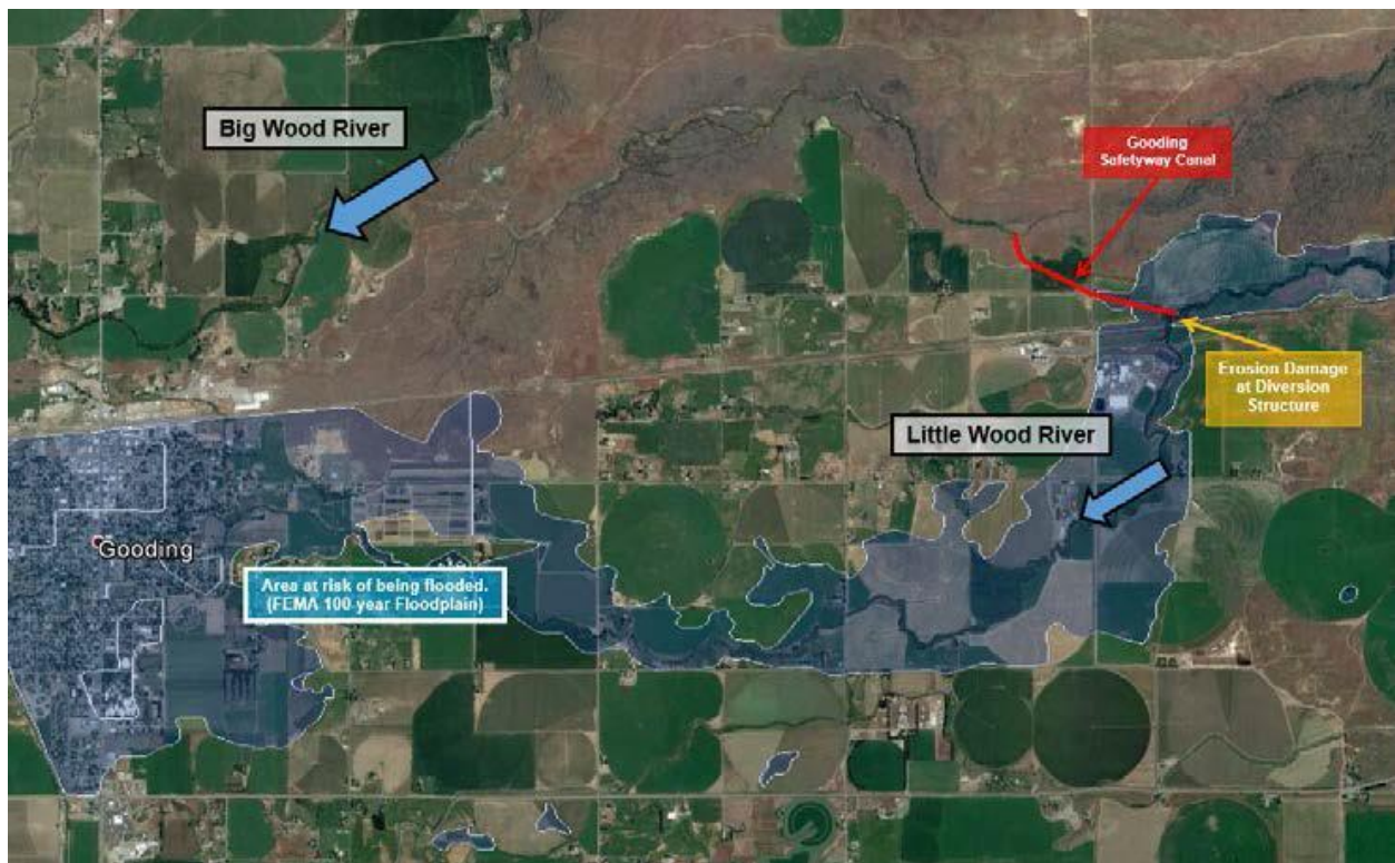
Figure 1-8. Gooding diversion structure, canal centerline, and area at risk of being flooded.
